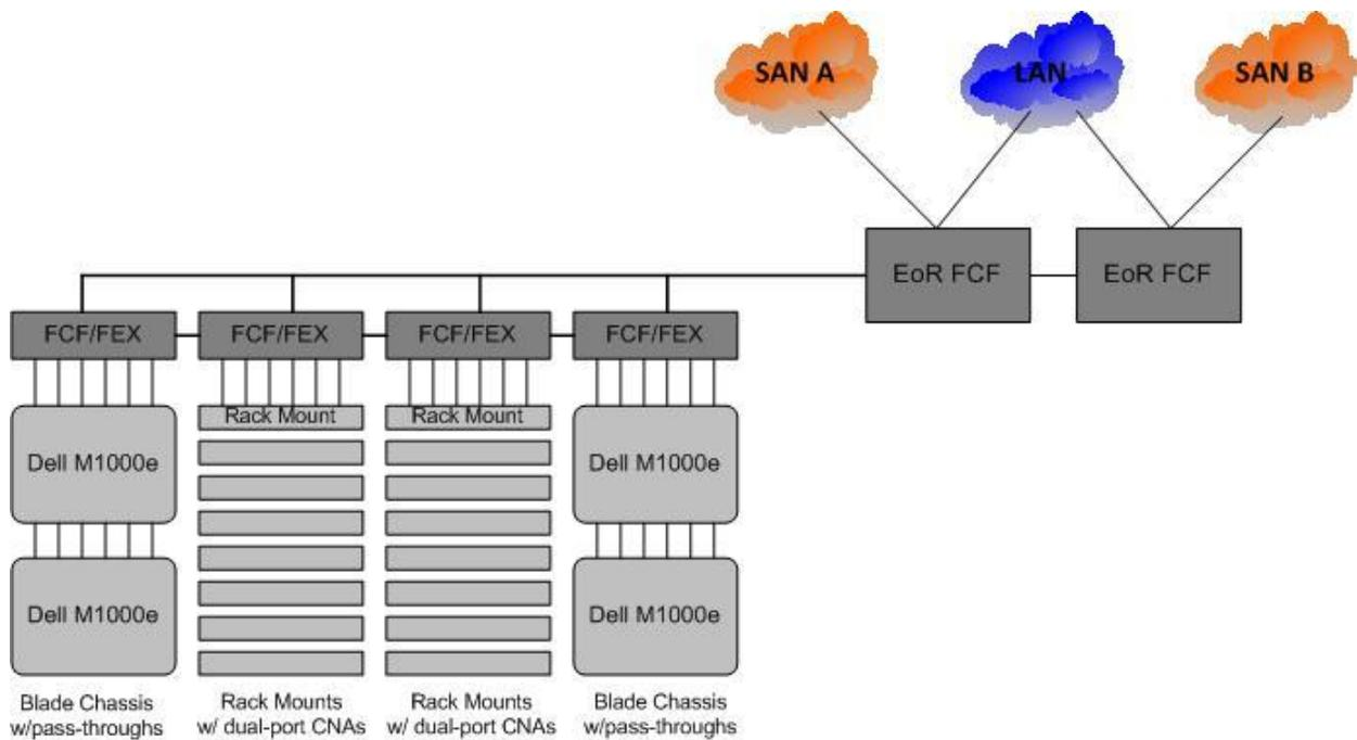
**Figure 1 Uniform Server Access Architecture**
