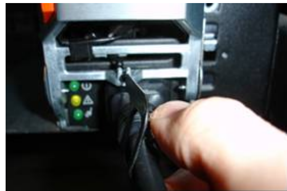
Figure 10b - Flip off retainer with thumb
