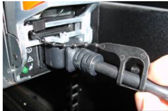
Figure 9d - Retainer clipped onto cord
