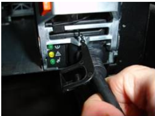
Figure 10c - Remove power cord from PSU
