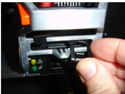
Figure 10e - Re-secure retainer to PSU handle
