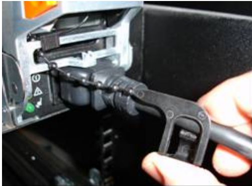
Figure 9c - Clip retainer onto cord
