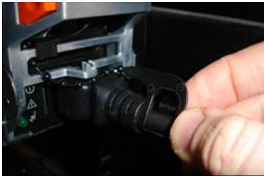
Figure 9e - Slide retainer against overmold
