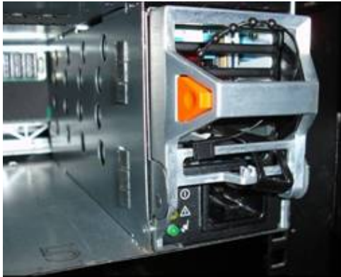
Figure 9a - Start with secured retainer
