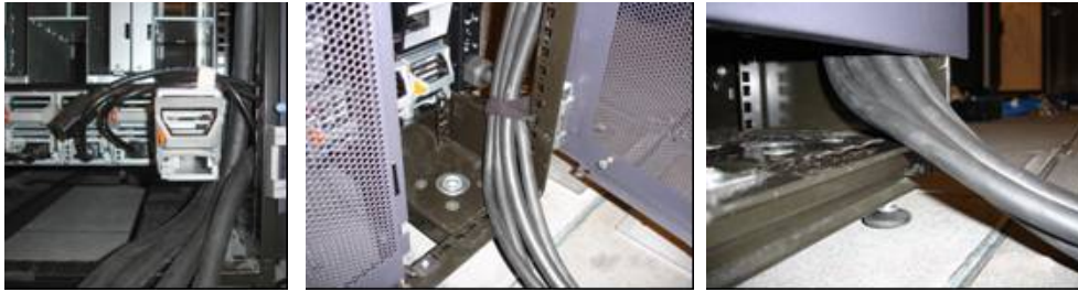
Figure 8 – Routing of inlet power cord around bottom corner PSU. Chassis is installed with a 2U gap underneath.
