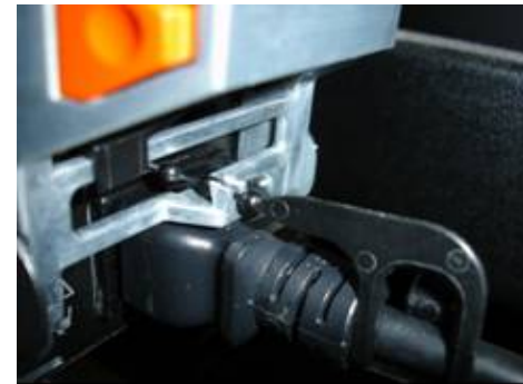
Figure 9f - Secure beaded tie into cleat on PSU handle
